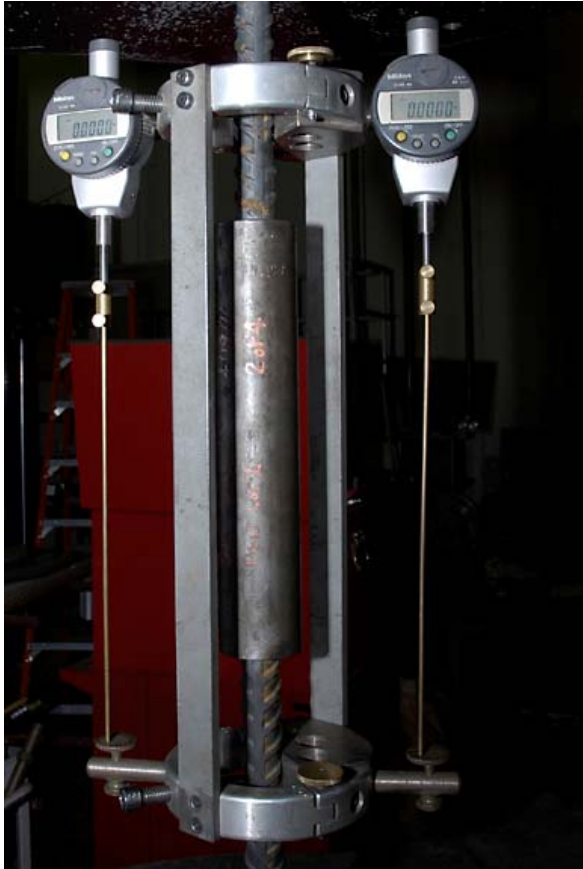
Figure 2b. Measuring device ready for testing with bottom hex socket bolts removed.
