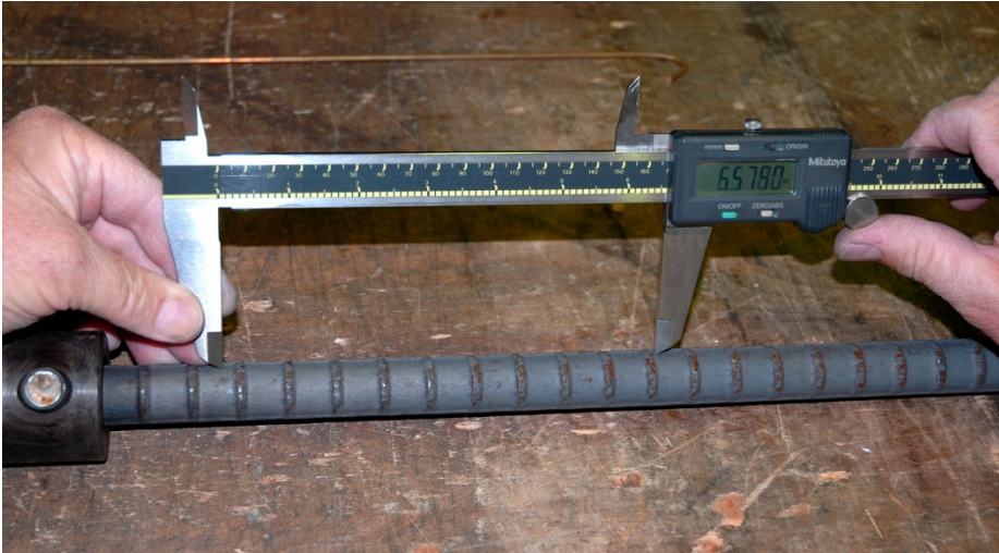
Figure 4. Digital calipers used to measure initial gage length to the nearest 0.001”.
