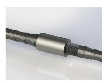
Barcoup L Couplers are designed to splice the same diameter bars where none of the bars can be rotated. The couplers are machined to have parallel threads inside which create a mechanical connection of two corresponding reinforcing steel. These rebars which will be connected are put together in site for mounting and the mounting is completed only by screwing the coupler by hand from right to left (with no need for extra torque wrench and controlling device).
