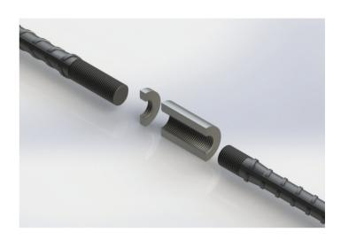
Poscoup Couplers are designed to splice the same diameter bars where at least one bar is not free to rotate. The couplers are machined to have parallel threads inside which create a mechanical connection of two corresponding reinforcing steel.
