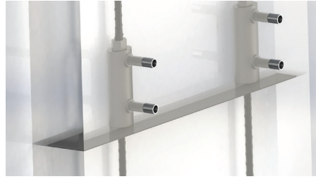
2. Align the corresponding precast element.
