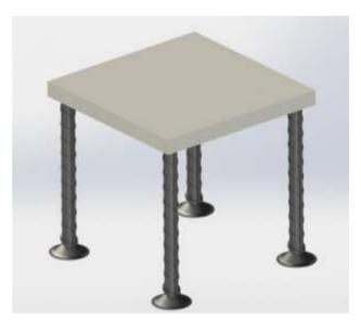
**Regbar Strong Anchor Plates** are designed to transfer heavy loads in the load-bearing structures of the concrete frame. **The headed rebar anchors of Regbar Strong Anchoring Plates** are optimized for easy installation, even in dense reinforcement. Connection plates are steel parts that are assembled before hardening of the concrete. The plates transfer the loads from the plate to concrete structure. Structural fixings are made by welding the steel plate.
