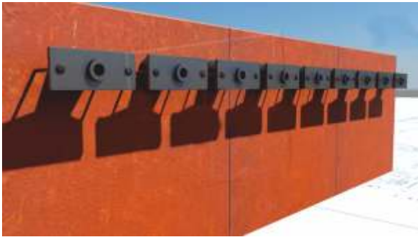
3) Plug the pocket former and anchorages to mold to get the tendon anchors
