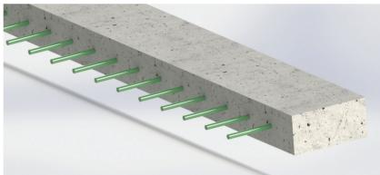
**4** Saw cut the slab over the centerline by diamond saw to a depth of 25 ~ 30% total slab thickness, as soon as it is possible to cut without damaging the arrises (within 24 hours). Control the depth of the cut to make sure the dowels are not cut through.
