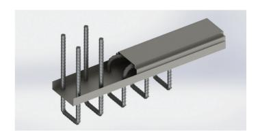
Regbar Rebend Connection system is used for effective connection of the concrete pieces which are poured and connected in different phases. The cover can be taken out of the body, thus it is manufactured from the galvanized sheet with the in-advanced drilled clutch holes and the protection system.
