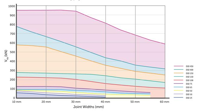
Regbar SSD  $V_{Rd}$  Design Resistance (kN) for Various Joint Widths (mm) at the Maximum Slab Thickness (mm) in C30/37 Concrete (See the following pages for details)
