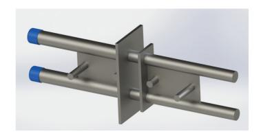
The Regbar SSD shear load connector is used where loads are small, but where alignment is critical. It is available in four sizes with each size available in two lengths. The dowel component is stainless steel bar.
