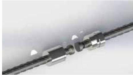
2. Align the corresponding rebar. Rotate the other part of coupler to create a mechanical connection.
