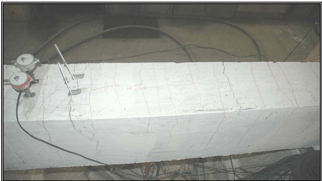
Figure 4.23 TS16 splice region after test.
