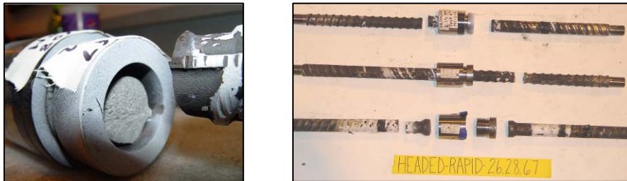
Figure 4. Post-test photos of upset head specimens tested at rapid strain-rate.
