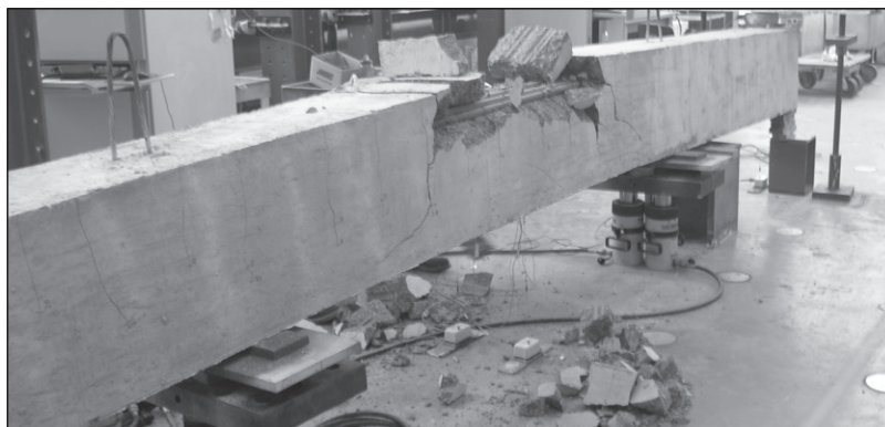
(a) Beams reinforced with No. 9 (28 mm diameter) bars
