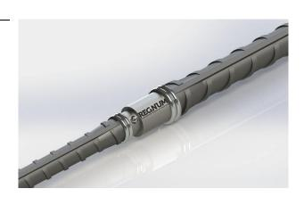
Friccoup Couplers are designed to splice the same diameter bars where at least one bar can be rotated and moved freely in its axial direction. Rotary Friction Welding (RFW) is a solid-state welding process that generates heat through mechanical friction between workpieces in relative rotation motion to one another, with the addition of a lateral force called "upset" to plastically displace and fuse the materials.
