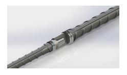
3. Align the corresponding rebar with female friccoup. Rotate the rebar until there is no further movement available between the two sections.
