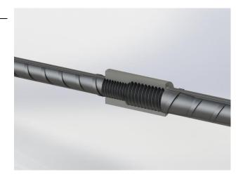
Transcoup Couplers are designed to splice different diameter bars where at least one bar can be rotated and moved freely in its axial direction. The couplers are machined to have parallel threads inside which create a mechanical connection of two corresponding reinforcing steel.
