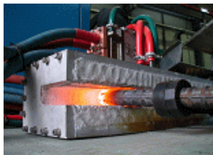
Fig. 2. Preheating the steel rebar section Fig. 3. Molding the preheated section
