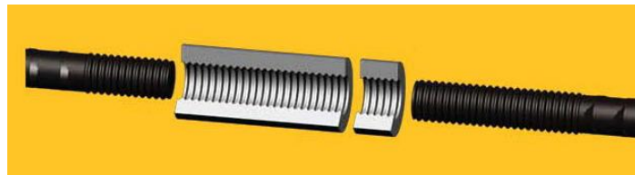
Figure 1. Schematic illustration of the Simgrip LT splice system. Note: product as tested did not include the locknut.
