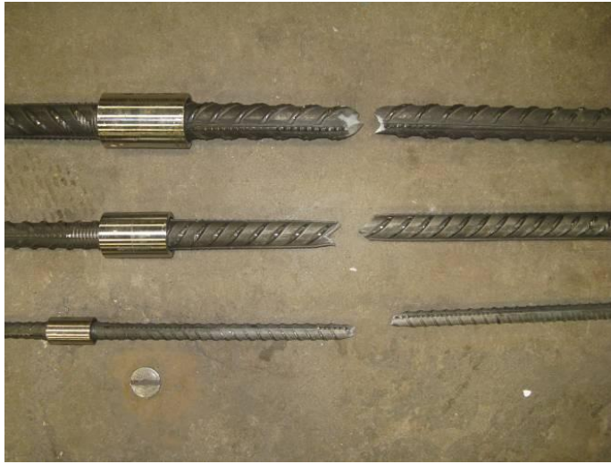
Figure 3. Representative fractured test specimens, showing bar break away from the mechanical splice
