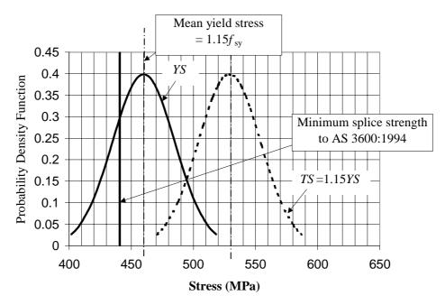
Fig. 1 Estimated strength of superseded Australian 400Y bar
