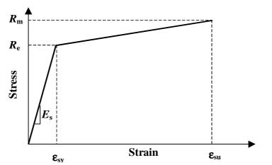
Fig. 3 Approximate stress-strain curve of new Australian 500N bar [3,6]
