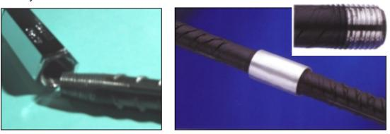
(a) Tapered thread cut into bar [8,9]
