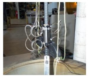
Fig. 7 Test set-up for measuring end slips and extension over coupler
