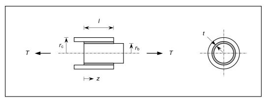
Fig. 9 Idealised theoretical model for one half of a threaded coupler
